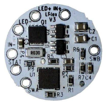
The picture shows the top of the LFlex. The user provides DC power to the LFlex (via battery, DC wallwart etc) via the IN+ (positive input voltage) and IN- (negative input voltage) pads.
