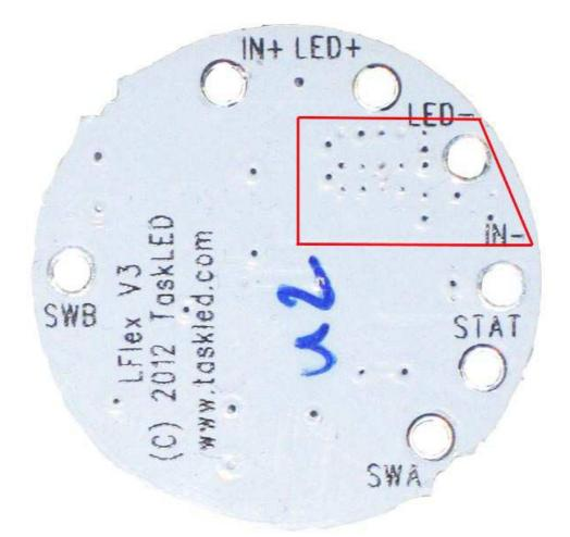
The red polygon encloses the minimum area that must be thermally coupled to the heatsink with the providec thermal pad material. It is preferential to mount the entire bottom area of the LFlex to a heatsink since the additional area will incrementally improve cooling.
