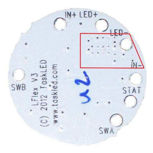
The red polygon encloses the minimum area that must be thermally coupled to the heatsink with the providec thermal pad material. It is preferential to mount the entire bottom area of the LFlex to a heatsink since the additional area will incrementally improve cooling.
